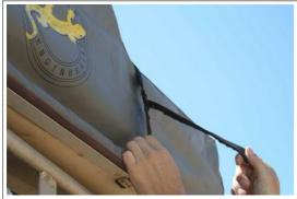
Tension the cover straps to avoid ballooning of the travel cover.
