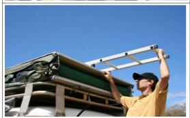
Slide out the ladder until the locking pins engage.
