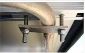
Tighten all the nuts and make sure your tent is securely fixed. The mounting plate should slightly bend around your rack.
